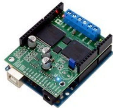
Pololu dual VNH5019 motor driver shield, assembled and connected to an Arduino Uno R3.
