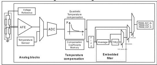
Figure 13. Hardware digital filter
