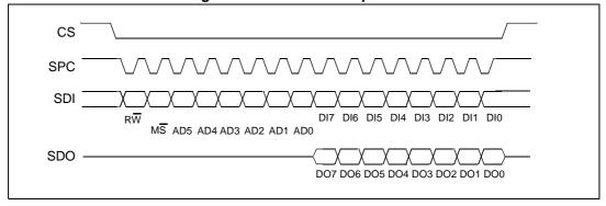
**CS** is the serial port enable and it is controlled by the SPI master. It goes low at the start of the transmission and returns to high at the end. **SPC** is the serial port clock and it is controlled by the SPI master. It is stopped high when **CS** is high (no transmission). **SDI** and **SDO** are respectively the serial port data input and output. Those lines are driven at the falling edge of **SPC** and should be captured at the rising edge of **SPC**.
