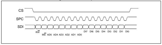
The SPI Write command is performed with 16 clock pulses. The multiple byte write command is performed adding blocks of 8 clock pulses at the previous one.
