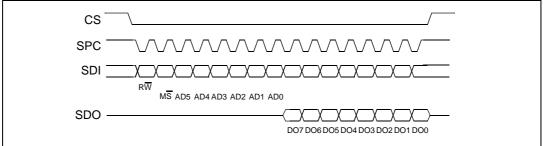
The SPI Read command is performed with 16 clock pulses. The multiple byte read command is performed adding blocks of 8 clock pulses at the previous one.
