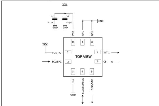
Figure 5. LPS25H electrical connection
