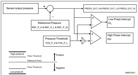
Figure 12. Interrupt generation block and output pressure data
