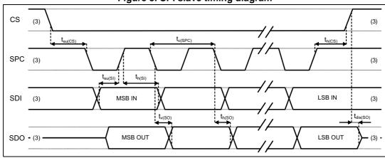
Figure 3. SPI slave timing diagram
