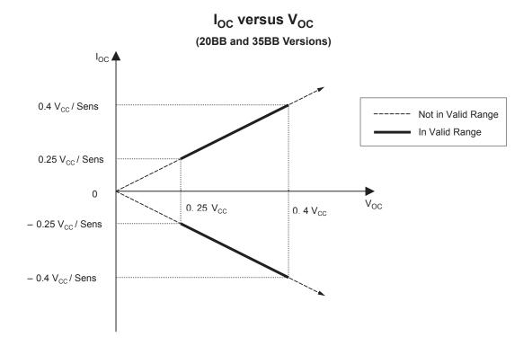
Example: For ACS709LLFTR-35BB-T, if required overcurrent fault switchpoint is 50 A, and  $V_{CC}$  = 5 V, then the required  $V_{OC}$  can be calculated as follows:
