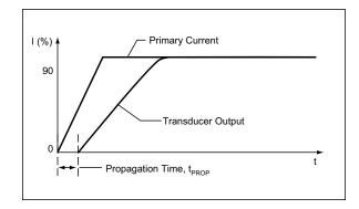
**Response time** ( $t_{RESPONSE}$ ). The time interval between a) when the primary current signal reaches 90% of its final value, and b) when the device reaches 90% of its output corresponding to the applied current.
