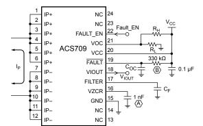
$\begin{array}{c|c} R_H,\,R_L & \text{Sets resistor divider reference for V}_{OC} \\ C_F & \text{Noise and bandwidth limiting filter capacitor} \\ C_{OC} & \text{Fault delay setting capacitor, 22 nF maximum} \\ \hline \langle A \rangle & \text{Use of capacitor required} \\ \hline \langle B \rangle & \text{Use of resistor optional} \\ \end{array}$
