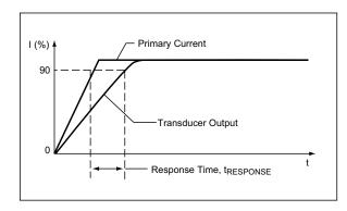
**Rise time** ( $t_r$ ). The time interval between a) when the device reaches 10% of its full scale value, and b) when it reaches 90% of its full scale value. The rise time to a step response is used to derive the bandwidth of the current sensor IC, in which  $f(-3 \text{ dB}) = 0.35/t_r$ . Both  $t_r$  and  $t_{RESPONSE}$  are detrimentally affected by eddy current losses observed in the conductive IC ground plane.
