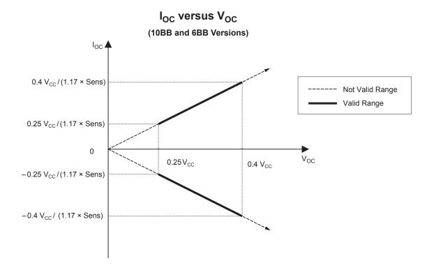
Example: For ACS709LLFTR-6BB-T, if required overcurrent fault switchpoint is 10 A, and  $V_{CC}$  = 3.3 V, then the required  $V_{CC}$  can be calculated as follows:
