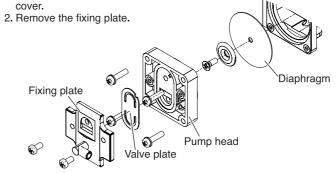
3. Clean the valve plate, fixing plate and pump head with isopropyl alcohol. Align the notch on the pump head with the corresponding notch on the valve plate.
