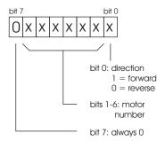
To obtain the complete byte 3 value from a motor number and a direction, multiply the motor number by 2 and add 1 if the direction is forward. For example, to make motor 5 go forward, byte three should be  $5 \times 2 + 1 = 11$ . To make motor 1 go backward, byte 3 should be  $1 \times 2 = 2$ . (Two efficient ways to multiply by 2 in a microcontroller program are shifting left by one digit or adding the motor number to itself.)
