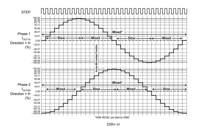
Figure 12: Decay Modes for Eighth-Step Increments
