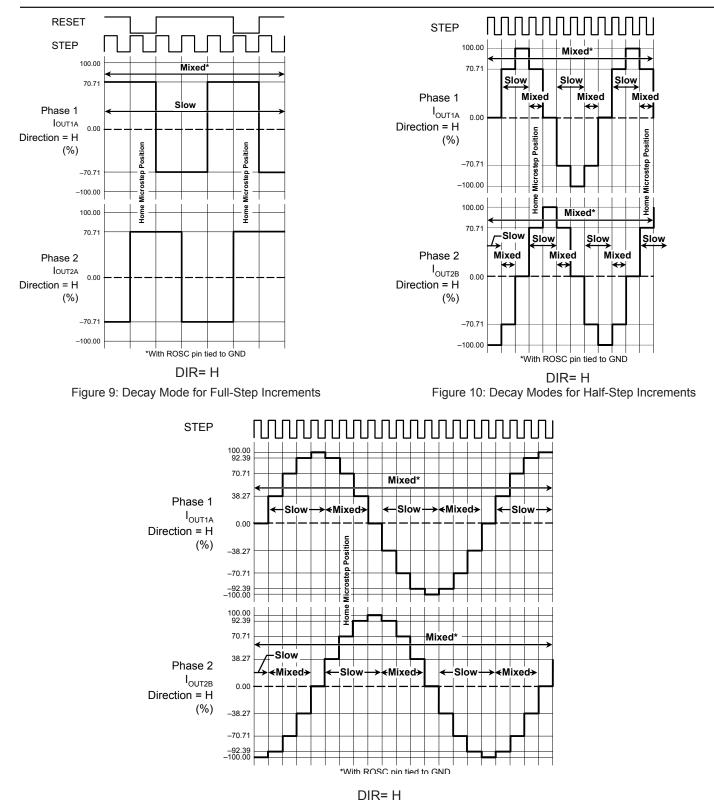
Figure 11: Decay Modes for Quarter-Step Increments
