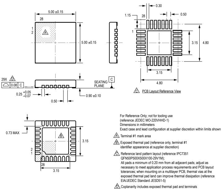
ET Package, 28-Pin QFN with Exposed Thermal Pad
