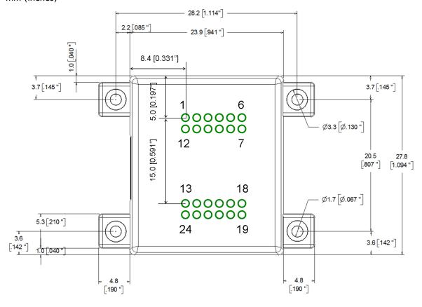
Part number 609-2890-ND from Digi-Key is a compatible 2mm pin header for connecting to the bottom connectors on the UM6.
