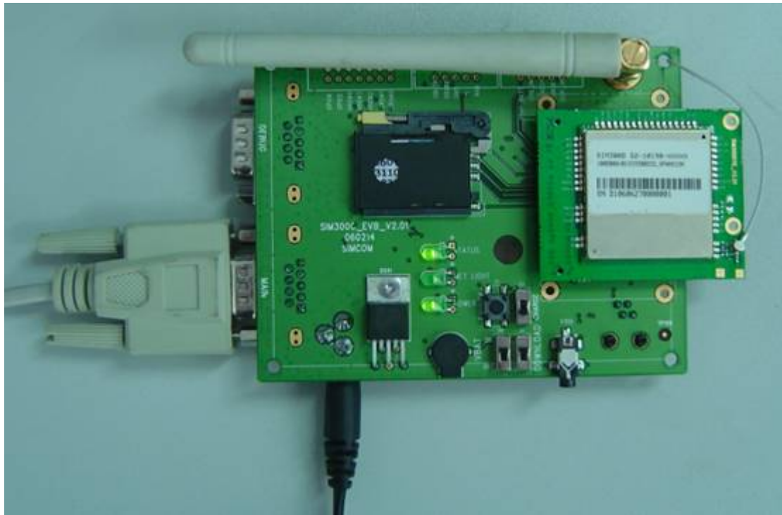
Figure 3: Top view of SIM3XXDZ EVB
