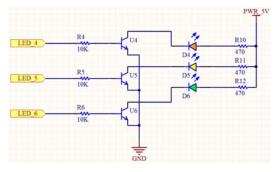
All LEDs are switched by transistors
