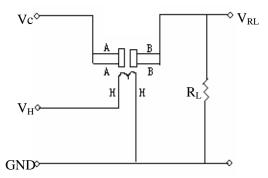
The above is basic test circuit of the sensor. The sensor need to be put 2 voltage, heater voltage(VH) and test voltage(VC). VH used to supply certified working temperature to the sensor, while VC used to detect voltage (VRL) on load resistance (RL) whom is in series with sensor. The sensor has light polarity, Vc need DC power. VC and VH could use same power circuit with precondition to assure performance of sensor. In order to make
