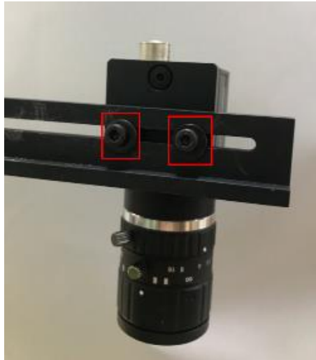
Figure 2.7 Fix camera mounting plate
