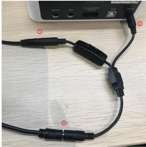
Figure 2.17 Connect light source switch
