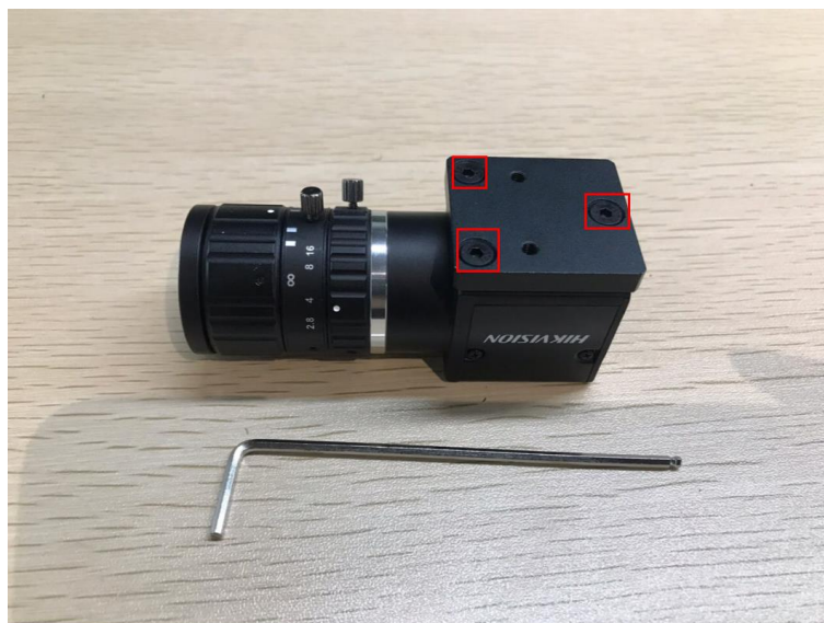
Figure 2.6 Fix camera plate
