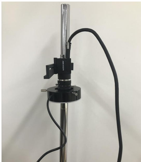
Figure 2.16 Fasten the light source kit
