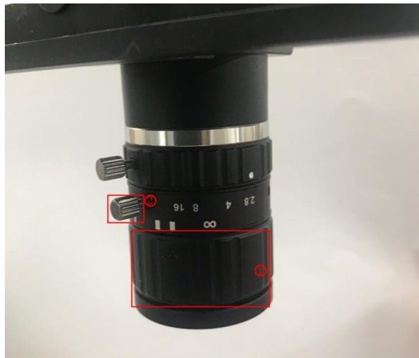
Figure 2.12 Adjust focal length
