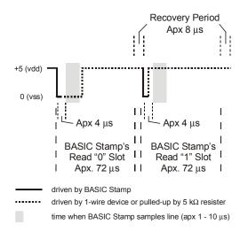
Figure 5.21: Example Read Slot.
