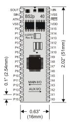
The BASIC Stamp 2p is available in the above two physical packages. Both packages use surface mount components to fit in a small package. The BS2p24-IC (Figure 1.9) is a 24-pin DIP package. The BS2p40-IC (Figure 1.10) is a 40-pin DIP package. Both packages are functionally equivalent accept that the BS2p40 has 32 I/O pins instead of 16.
