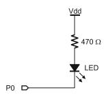
Figure 5.30: LED Circuit for PULSOUT Demo Programs.
