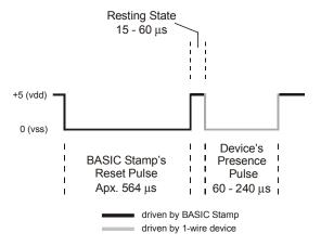
This reset pulse is controlled by the lowest two bits of the *Mode* argument in the OWIN command. It can be made to appear before the ROM Function Command (ex: Mode = 1), after the Transaction/Data portion (ex: Mode = 2), before and after the entire transaction (ex: Mode = 3) or not at all (ex: Mode = 0). See the section on Mode, above, for more information.
