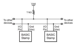
**Figure 5.40:** SEROUT Open-Drain Circuit. This circuit is for use with the Open, Non-inverted baudmode.
