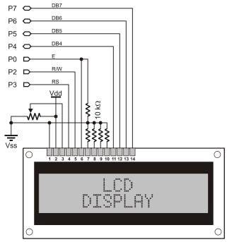
Figure 5.14: Example LCD Circuit. Shown with all connections necessary for the LCDCMD, LCDIN and LCDOUT commands.
