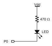
**Figure 5.45:** SLEEP Example LED Circuit.
