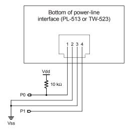
Figure 5.48: XOUT Power-Line Interface Circuit.
