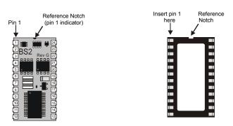
**Figure 1.13:** Pin 1 Indicators BS2-IC shown in the correct orientation in relation to a 24-pin socket.
