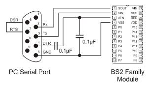
**Figure 1.16:** Programming and Run-time Communication Connections for all BS2 models.
