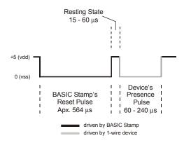
This reset pulse is controlled by the lowest two bits of the *Mode* argument in the OWOUT command. It can be made to appear before the ROM Function Command (ex: Mode = 1), after the Transaction/Data portion (ex: Mode = 2), before and after the entire transaction (ex: Mode = 3) or not at all (ex: Mode = 0). See the section on Mode, above, for more information.
