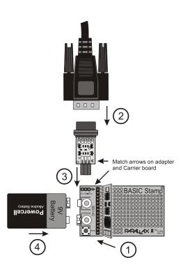
Figure 2.1: BS1-IC, BS1 Carrier Board, and BS1 Serial Adapter
