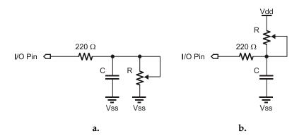
Figure 5.33: Example RC Circuits. Use a (left) with State = 1. Use b (right) with State = 0.
