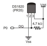
Figure 5.26: DS1820 Circuit. NOTE: The 4.7 k $\Omega$  resistor is required for proper operation.
