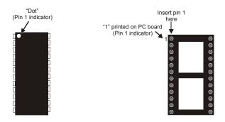
Figure 1.14: Additional Examples of Pin 1 Indicators (chip and socket shown in the correct orientation in relation to each other)
