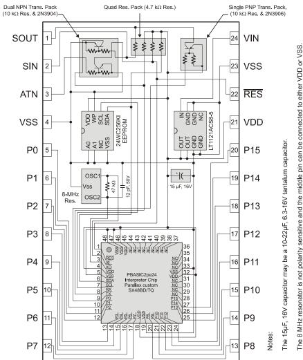
The 8 MHz resonator is not polarity sensitive and the middle pin can be connected to either VDD or VSS.
