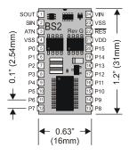
**Figure 1.5:** BASIC Stamp 2 OEM (Rev. A2) (Stock# 27290 assembled, or #27291 in kit form).
