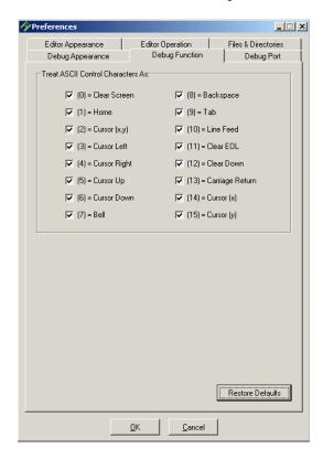
Figure 3.25: The Debug Function Tab under Edit  $\rightarrow$  Preferences.
