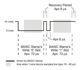
Figure 5.25: Example Write Slots.
