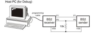
**Figure 5.37:** Flow-Control Example Circuit.
