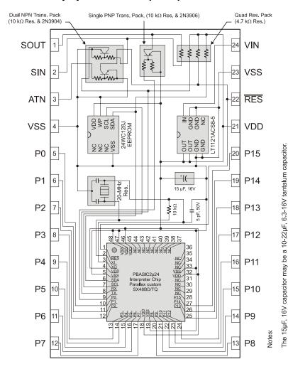
The 20 MHz resonator is not polarity sensitive and the middle pin can be connected to either VDD or VSS.
