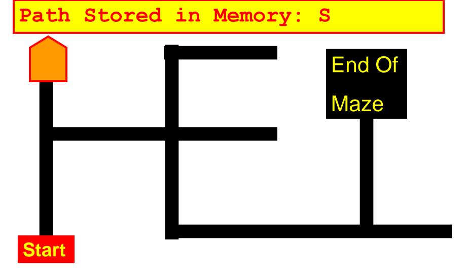
The robot runs off the path (Pattern = "00000") and the correct behavior is to take a U-Turn.
