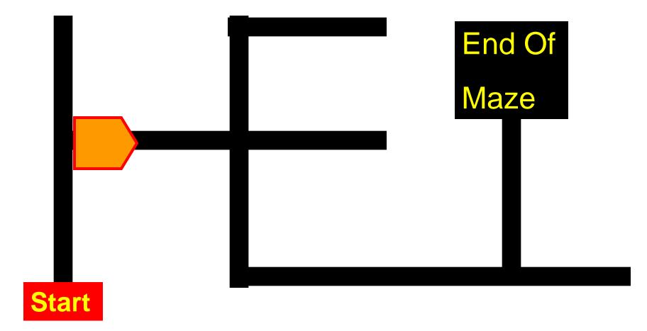
What could the robot have done to avoid going down the dead-end path? Instead of "SUL", the robot should have done "R".
