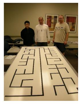
Each line maze has a Start point and a Finish point. The robot is expected to follow the lines and find it's way from Start to Finish in the fastest time possible.
