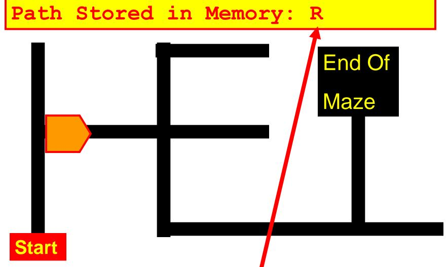
And replace "SUL" with "R". This tells the robot, next time through the maze, to take a right turn at the first intersection.
