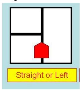
If the sensor pattern is now "00000", then the robot is at a "Left Turn Only". With any other reading, the robot is at the "Straight or Left" intersection.
