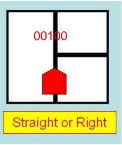
If the sensor pattern is now "00000", then the robot is at a "Right Turn Only". With any other reading, the robot is at the "Straight or Right" intersection.
