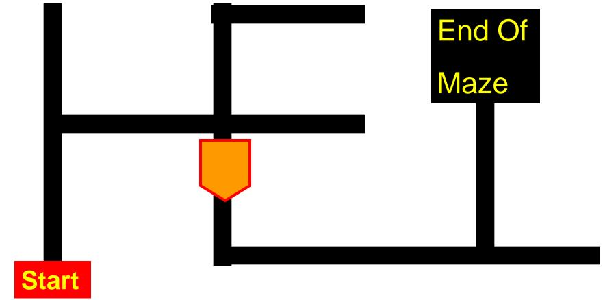
We got here with "SUL", so the correct path next time will be to take a right turn, so replace "SUL" with "R".
