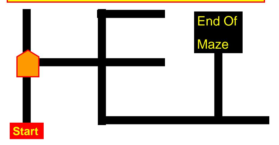
The robot takes off! At the first intersection, the robot senses a "Straight or Right" intersection. The left hand rule requires that the robot go straight.
