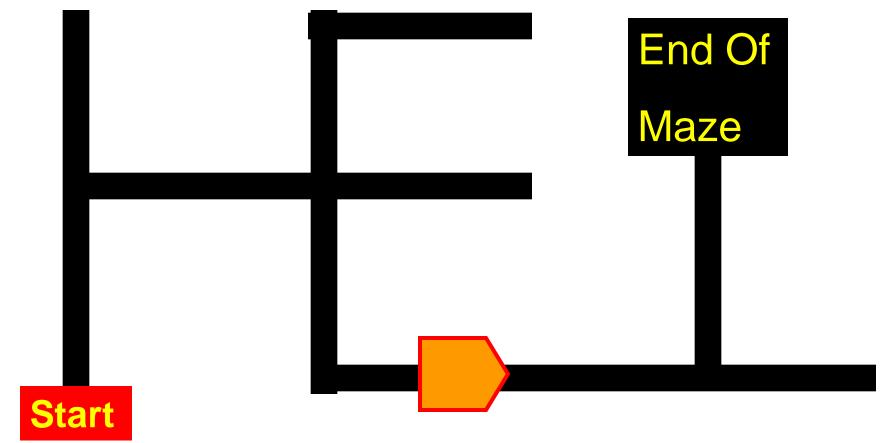
Only one more turn! The intersection coming up is a "Straight-Left" and the left hand rule will have the robot turn left and record an "L".
