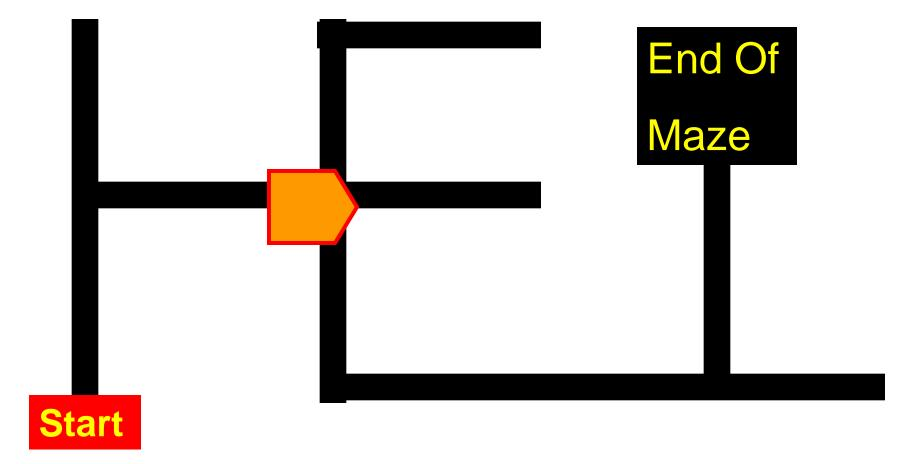
The next intersection is a "Four-Way" Intersection. The left hand rule requires a left hand turn, so turn left and record an "L".
