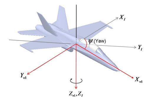
Figure 2 - The Vehicle-1 Frame.
