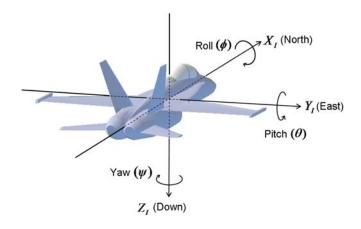
Attitude and Heading Sensors from CH Robotics can provide orientation information using both Euler Angles and Quaternions. Compared to quaternions, Euler Angles are simple and intuitive and they lend themselves well to simple analysis and control. On the other hand, Euler Angles are limited by a phenomenon called "Gimbal Lock," which we will
