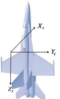
An orientation sensor or AHRS that uses Euler Angles will always fail to produce reliable estimates when the pitch angle approaches 90 degrees. This is a fundamental problem of Euler Angles and can only be solved by switching to a different representation method. All CH Robotics attitude sensors use quaternions so that the output is always valid even when Euler Angles are not.
