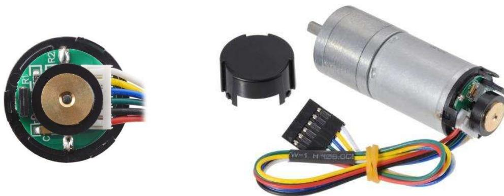
The quadrature encoder provides a resolution of 48 counts per revolution (CPR) of the motor shaft when counting both edges of both channels. To compute the counts per revolution of the gearbox output, multiply the gear ratio by 48.
