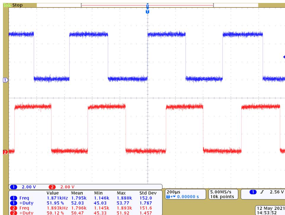
Counting both the rising and falling edges of both the A and B outputs results in 48 counts per revolution of the motor shaft. Using just a single edge of one channel results in 12 counts per revolution of the motor shaft, so the frequency of the A output in the above oscilloscope capture is 12 times the motor rotation frequency.
