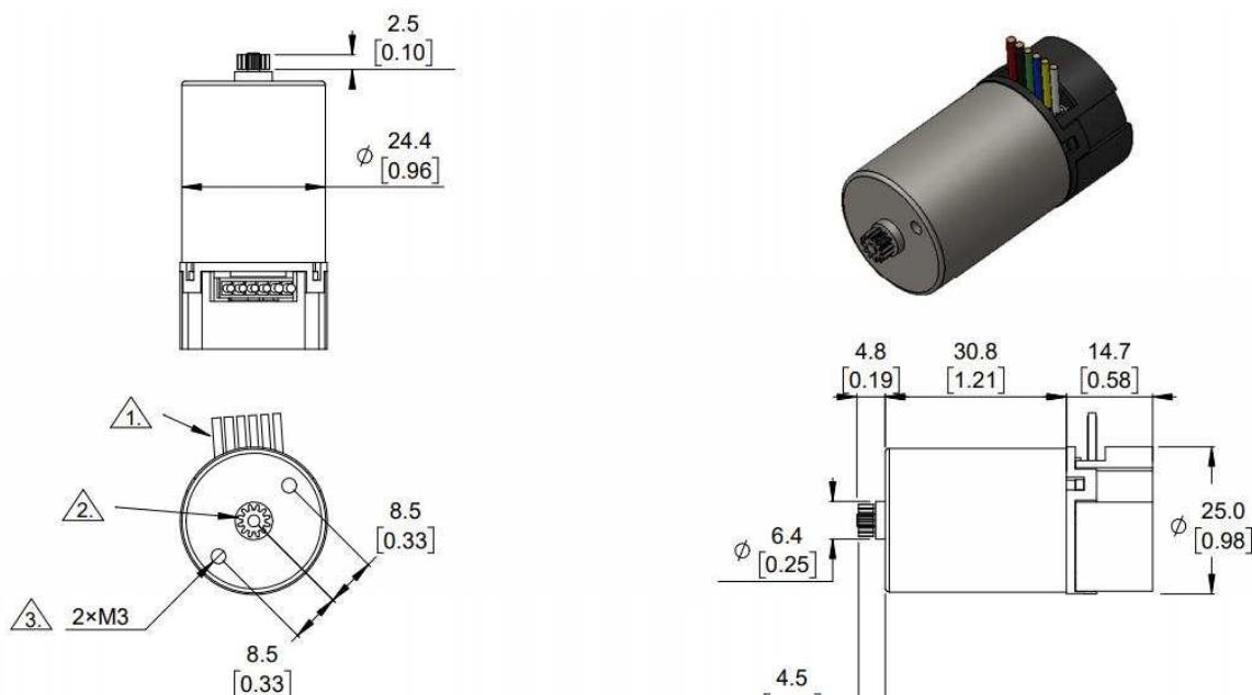
**1.** Leads are approximately 200 mm [8 in] long and are terminated by a 1x6 female header with a 2.54 mm [0.1 in] pitch.
