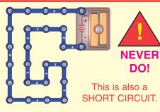
When the slide switch (S1) is turned on, this large circuit has a SHORT CIRCUIT path (as shown by the arrows). The short circuit prevents any other portions of the circuit from ever working.
