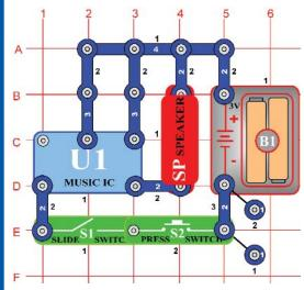
OBJECTIVE: To build an AND gate.
