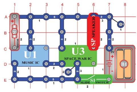
**OBJECTIVE:** To build a circuit that uses a motor to activate space war sounds.
