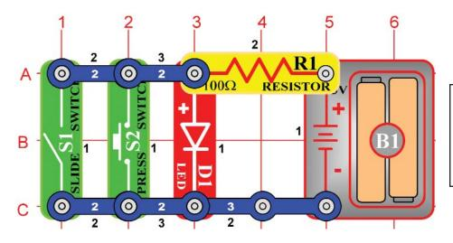
Build the circuit at left and test the combinations of the slide switch (S1) and press switch (S2). If you compare it to the OR circuit in Project #47, you can see the LED lights in the opposite combinations of that circuit. Hence, we refer to it as a <u>NOR</u> circuit (short for "NOT this OR that"). Like the OR and AND, it is an important building block in computers.
