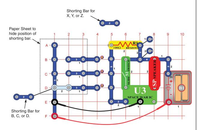
Build the circuit at left. It uses both jumper wires as permanent connections. It also uses two 2-snap wires as "shorting bars".
