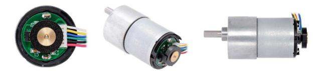
The quadrature encoder provides a resolution of 64 counts per revolution (CPR) of the motor shaft when counting both edges of both channels. To compute the counts per revolution of the gearbox output, multiply the gear ratio by 64.
