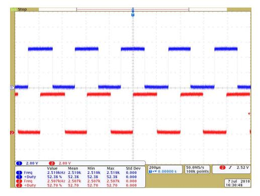
By counting both the rising and falling edges of both the A and B outputs, it is possible to get 64 counts per revolution of the motor shaft. Using just a single edge of one channel results in 16 counts per revolution of the motor shaft, so the frequency of the A output in the above oscilloscope capture is 16 times the motor rotation frequency.
