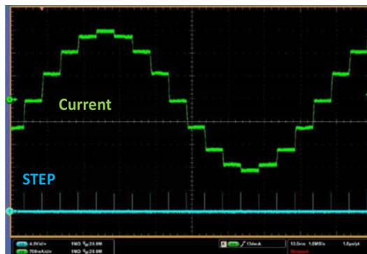
**Figure 1. Fixed-Off-Time PWM Chopping Illustration**
