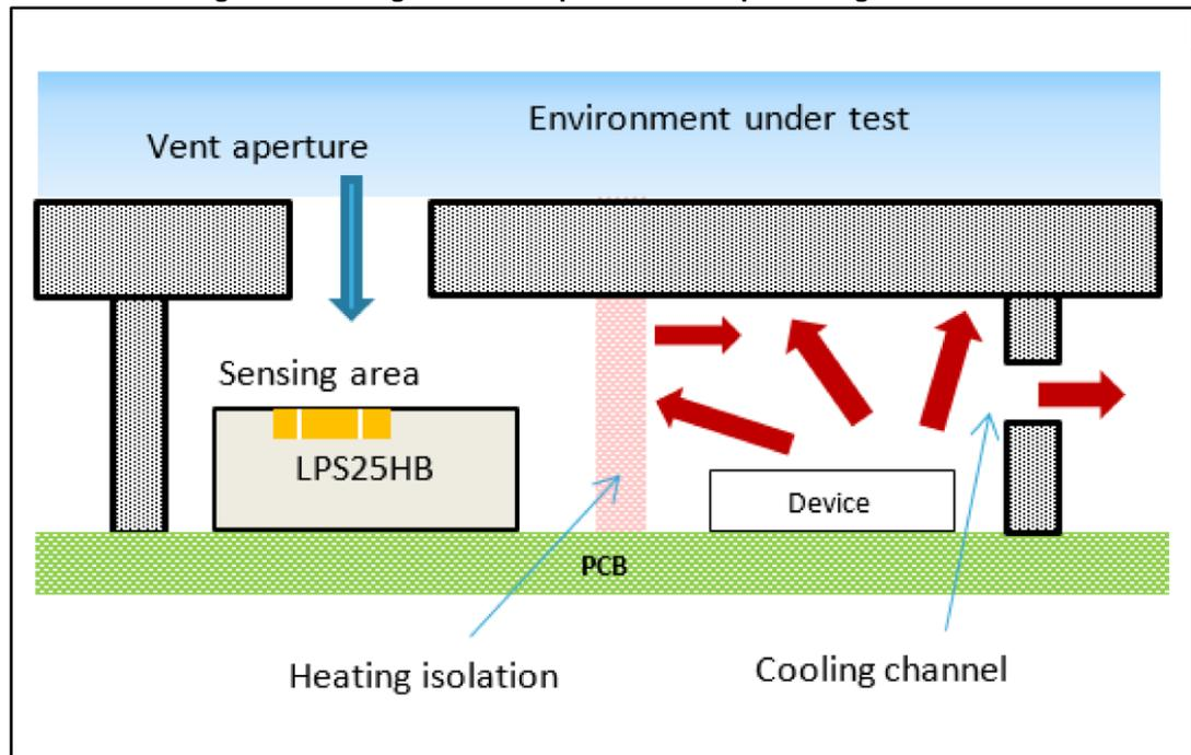
Looking at a section of the sensor housing, [Figure 5: "Top view of the sensor housing: on the left a correct design with the heat isolation, on the right a wrong design"](#) shows a good design with the heating isolation structure on the left; the heat source is far from the sensor and a thermal protection structure is placed in the middle. On the right, a wrong design is described, determining the sensor heating because of the heat radiation coming from the component nearby.
