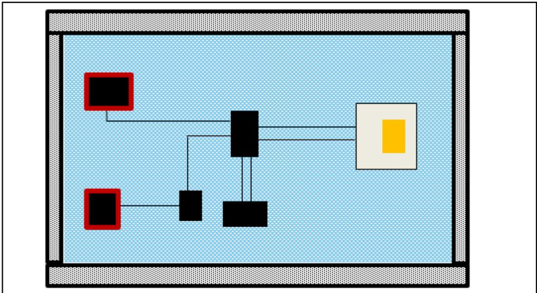
Figure 7: Sensor with a bad wiring on the PCB
