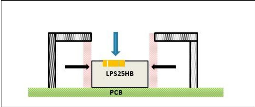
Figure 10: Bad configuration for mechanical stress (b)
