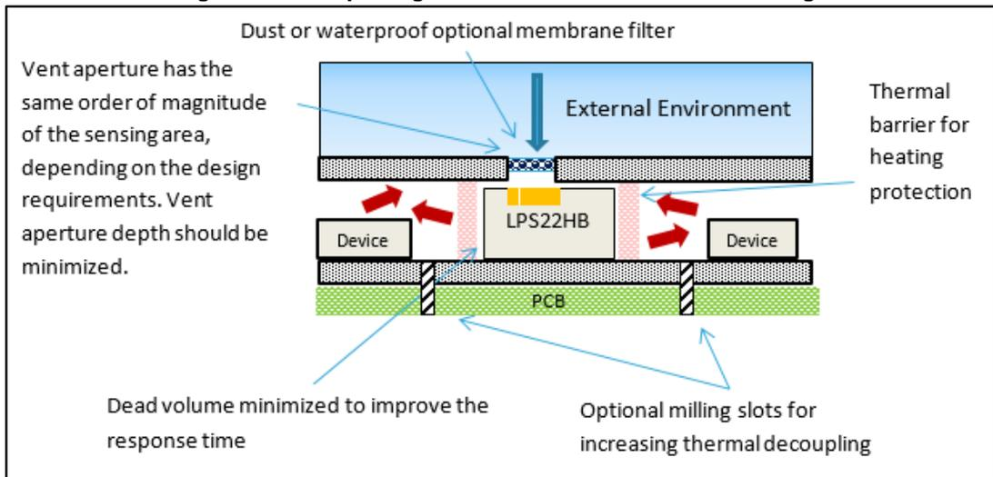
Figure 14: Example of good sensor embodiment and housing with airflow channel
