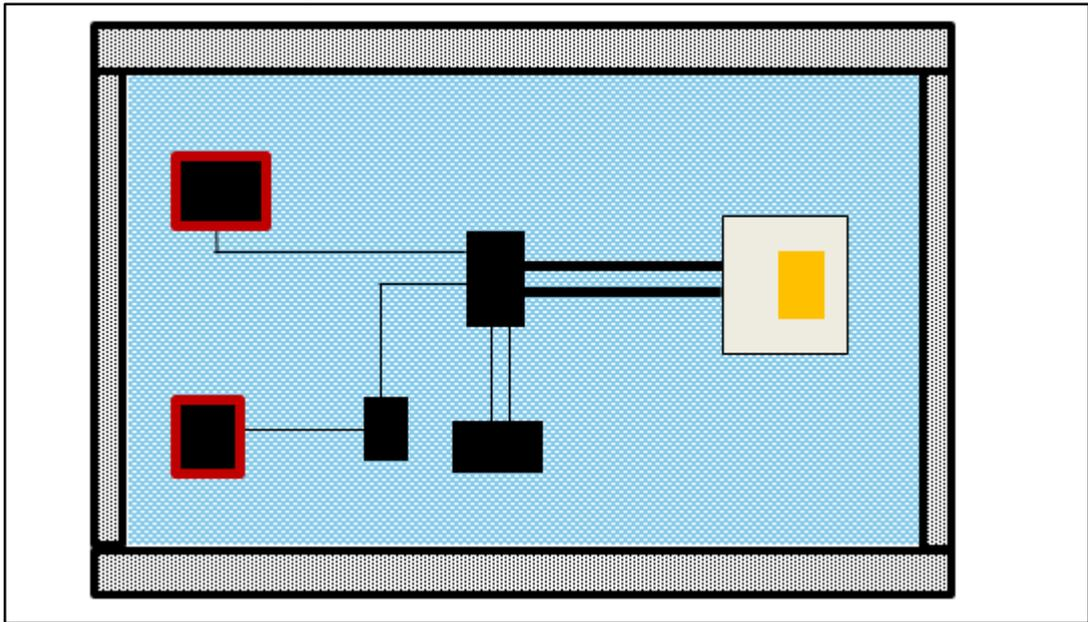
In *Figure 7: "Sensor with a bad wiring on the PCB"* a wrong metal lines size is adopted, the bigger dimensions will provide higher level of heating conduction. In *Figure 8: "Sensor wiring with wrong placement on the PCB"*, the wrong placement of the sensor, close to a device generating too much heating deteriorates the sensor performance.
