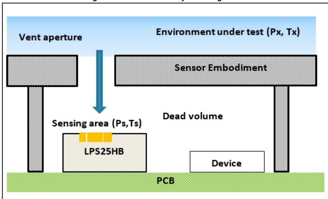
Therefore, in order to get a reliable and consistent measurement, all the parameters involved in the mechanical design must be dimensioned to get the maximum sensor exposition to the external environment, to get a faster response time, in terms of pressure and temperature, compatible with the required design specifications.
