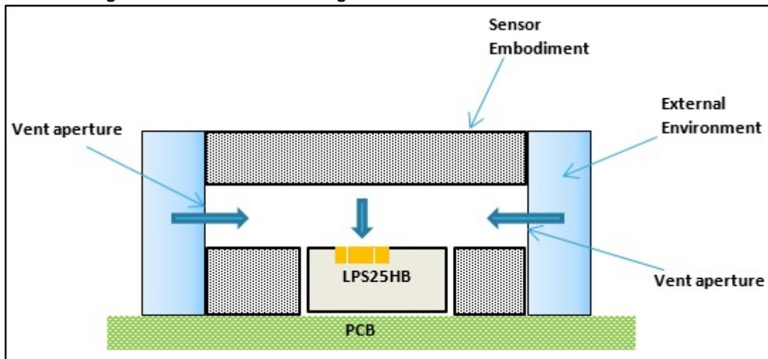
It is useful to underline that the sensor can work properly even if it is placed in customer's application system without considering any dedicated hole (vent aperture) unless that one is not hermetically sealed. The design guidelines reported above are for getting out top performances.
