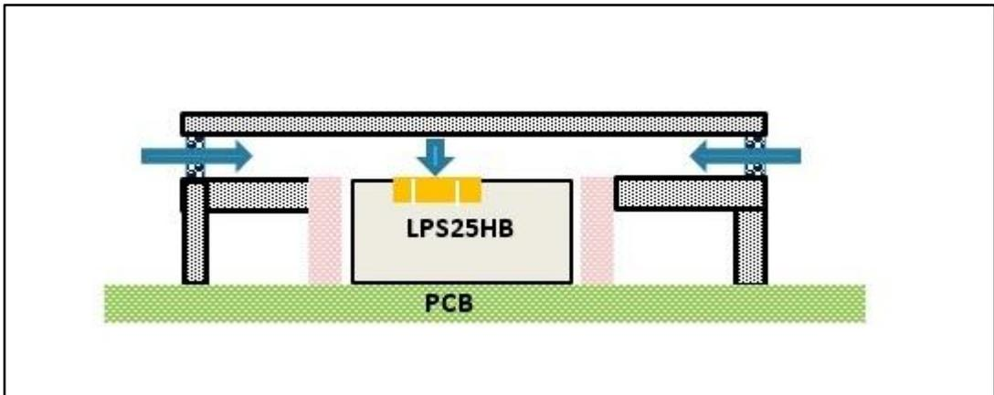
Figure 12: Good configuration for avoiding mechanical stress and reducing the dead volume (b)
