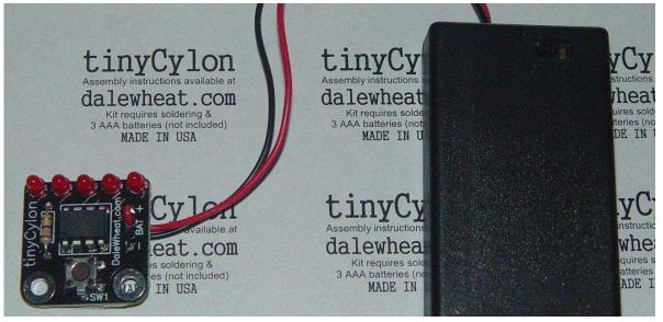
Photo 3. The assembled tinyCylon kit in the "classic" configuration, with all parts on one side. The battery holder is installed in the next step.
