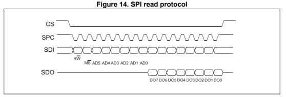
The SPI read command is performed with 16 clock pulses. The multiple byte read command is performed by adding blocks of 8 clock pulses to the previous one.
