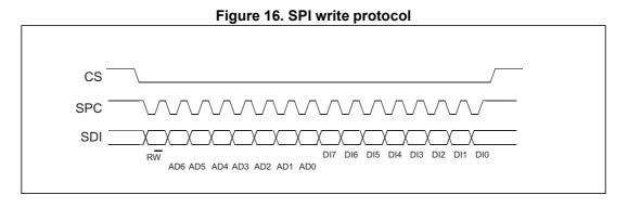
The SPI write command is performed with 16 clock pulses. The multiple byte write command is performed by adding blocks of 8 clock pulses to the previous one.
