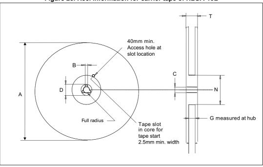
Figure 25. Reel information for carrier tape of HLGA-10L
