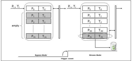
Figure 10. Bypass-to-Stream mode
