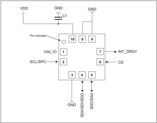
Figure 12. LPS25HB electrical connections (top view)
