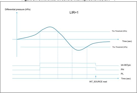
Figure 21. Differential threshold interrupt behavior, LIR = 1
