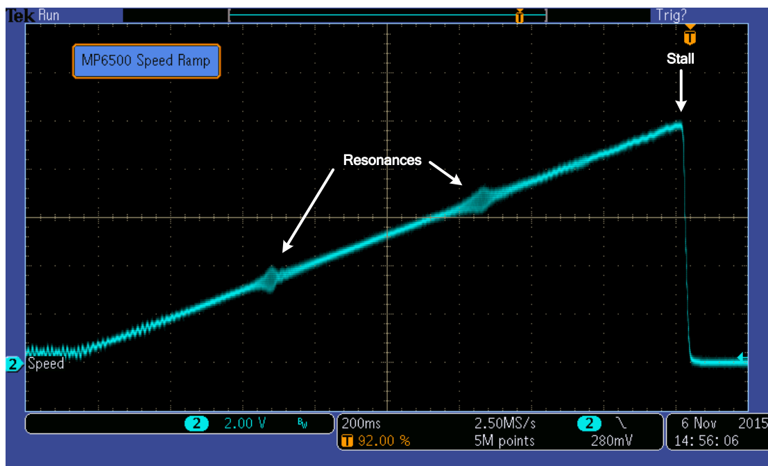
Figure 15: MP6500 Speed Ramp
