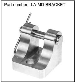
This bracket is tested to 1,265 lbs., which is 125% of the highest static load that Concentric International's Medium Duty line of actuators are rated for.
