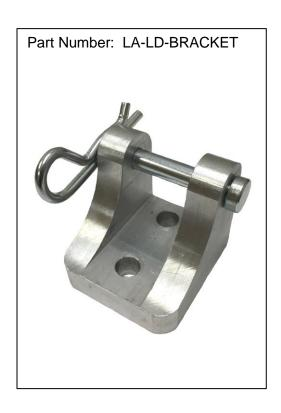
This bracket is tested to 703 lbs., which is 125% of the highest static load that Concentric International's Light Duty line of actuators are rated for.
