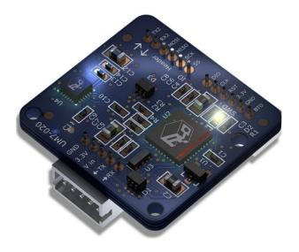
The UM7 is a 3rd-generation Attitude and Heading Reference System (AHRS) that takes advantage of state-of-the-art MEMS teschnology to improve performance and reduce costs. Like its predecessors, the UM7 combines triaxial accelerometer, rate gyro, and magnetometer data using a sophisticated Extended Kalman Filter to produce attitude and heading estimates.
