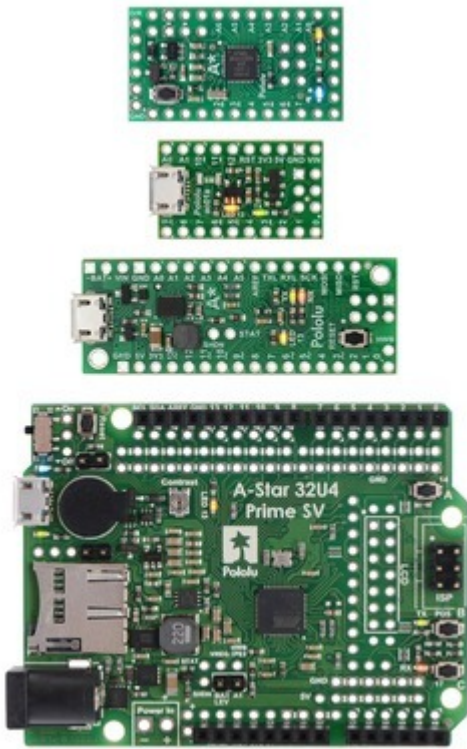
From top to bottom: A-Star 328PB Micro, 32U4 Micro, 32U4 Mini SV, and 32U4 Prime SV.
