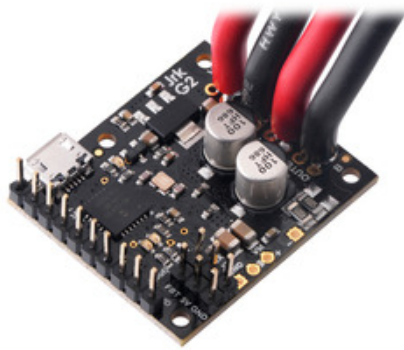
Jrk G2 18v19 or 24v13 USB Motor Controller with thick wires and included headers soldered.
