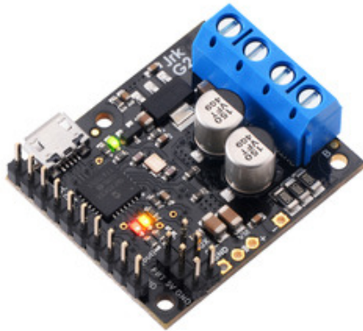
Jrk G2 18v19 or 24v13 USB Motor Controller with included terminal blocks and headers soldered.
