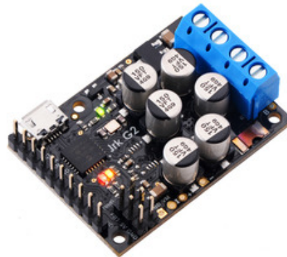
Jrk G2 18v27 or 24v21 USB Motor Controller with included terminal blocks and headers soldered.
