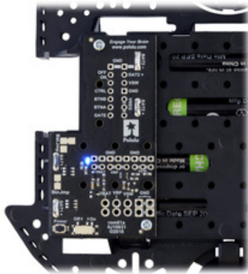
Power Distribution Board for Romi Chassis on a black chassis.
