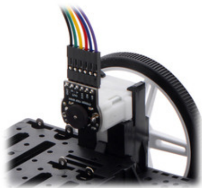
The included low-profile headers are still long enough to work with our pre-crimped jumper wires.
