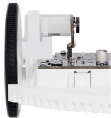
The Romi Encoder can plug directly into the Motor Driver and Power Distribution Board for Romi Chassis.
