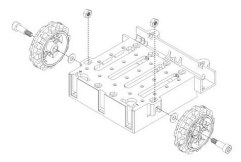
3. Insert the shoulder bolts through the side of the chassis into the nut. Use a 3 mm hex key (Allen wrench) to tighten the bolts until the washers are snug against the chassis. <u>Be careful not to overtighten the shoulder bolts</u> as doing so can bend the washers.
