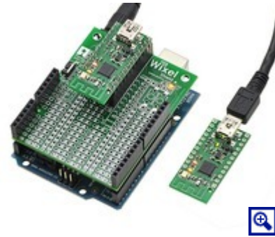
Wixel shield for Arduino powered through its power jack, communicating wirelessly with another Wixel.
