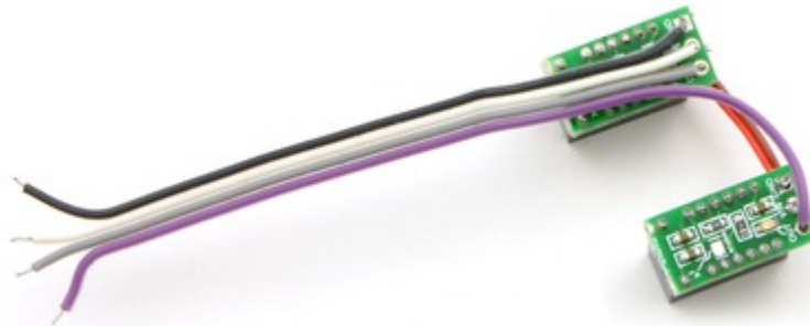
Soldering the sensors to a four-pin cable.
