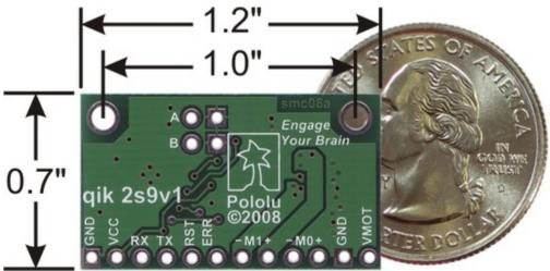
The qik 2s9v1 measures 0.7" x 1.2" x 0.28" (17.8 x 30.5 x 7.1 mm) and weighs 0.07 oz (2.0 g) without the header pins installed. It has two mounting holes, one in each top corner. The holes have a diameter of 0.086" and are designed for #2 or M2 screws.
