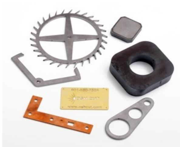
**Various metal parts cut by OSH Cut Laser Cutting.**
