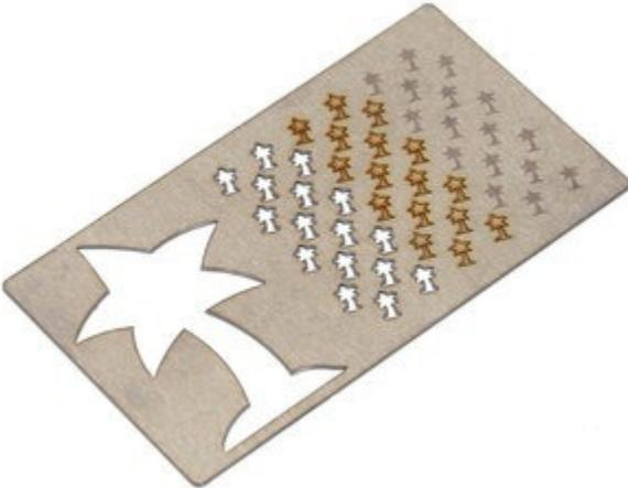
**Through-cutting, vector etching, and raster engraving on mild steel.**
