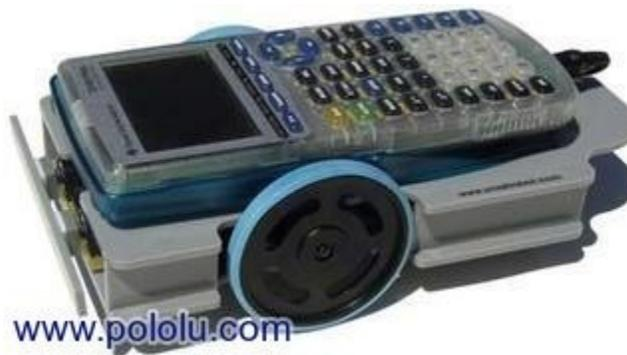
**Norland Research** [<http://www.smallrobot.com/>] manufactures a robot based on a graphing calculator, which has a chassis that is a good example of what can be made with a laser cutter. The dimensions of this chassis are designed to fit a Texas Instruments graphing calculator on the top level and the electronics, batteries, and servos on the bottom level. A similar design could be used for any basic robot.
