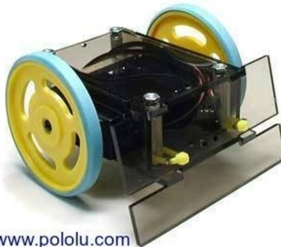
This custom sumo robot chassis is propelled by two radio-control hobby servos modified for
