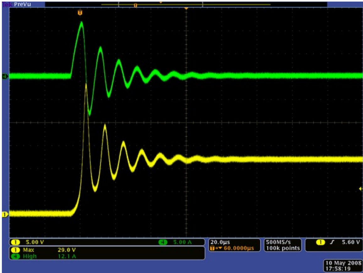
Oscilloscope capture of voltage (yellow) and current (green) when “double-clicking” a Pololu pushbutton power switch connected to a bench power supply.
