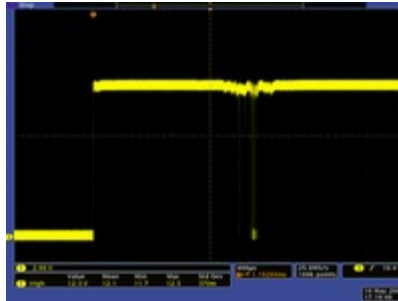
Oscilloscope capture of the output voltage of a small mechanical switch as it bounces.
