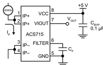
Application 1. The ACS715 outputs an analog signal,  $V_{OUT}$ , that varies linearly with the unidirectional DC primary sampled current,  $I_P$ , within the range specified.  $C_F$  is recommended for noise management, with values that depend on the application.
