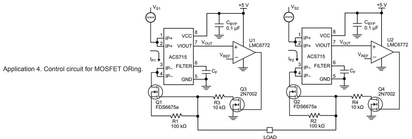
Application 4. Control circuit for MOSFET ORing.
