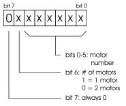
number and the one above it; if you set an odd motor number, the motor controller will control that motor number and the one below it. Note that all motor controllers will respond to motor number 0 (and 1, if in two-motor mode).
