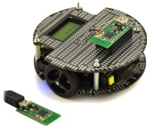
Wireless PC control of a 3pi robot using a pair of Wixels.
