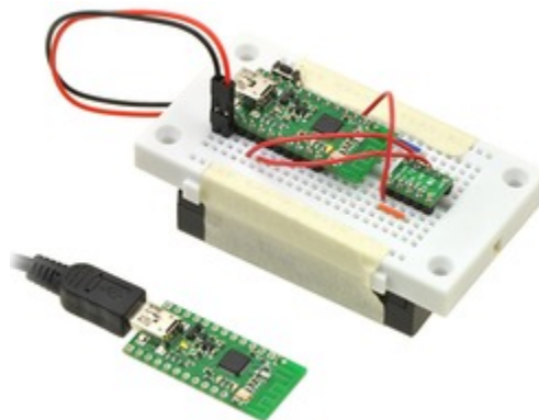
Wireless tilt mouse made with two Wixels and an accelerometer.
