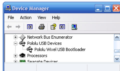
Windows XP Device Manager showing a Wixel in bootloader mode.
