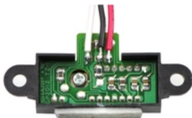
Sharp distance sensor with connected wires and double sided tape.
