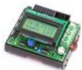
**Pololu Orangutan LV-168** [<https://www.pololu.com/product/775>]: a full-featured, mega168-based robot controller that includes an LCD display. The LV-168 runs on an input voltage of 2-5V, allowing two or three batteries to power a robot.
