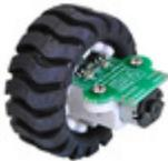
**Encoder for Pololu Wheel 42×19 mm** [<https://www.pololu.com/product/1217>]: a wheel encoder solution that allows a robot to measure how far it has traveled.
