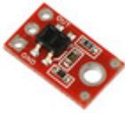
**Pololu QTR-1A** [<https://www.pololu.com/product/958>] and **QTR-8A** [<https://www.pololu.com/product/960>] **reflectance sensors (analog)**: an analog sensor containing IR/phototransistor pairs that allows a robot to detect the difference between shades of color. The QTR sensors can be used for following lines on the floor, for obstacle or drop-off (stairway) detection, and for various other applications.
