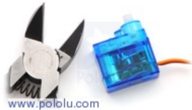
A sub-micro servo with mounting tabs clipped off.
