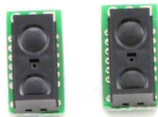
Digital distance sensors with trimmed carrier boards.
