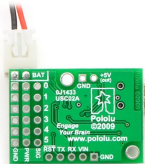
Soldering a power connector to the Micro Maestro.
