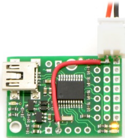
Self power and a battery connector on the Micro Maestro.
